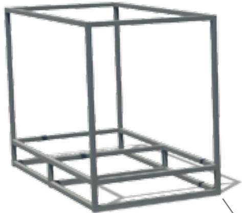
Each module has a steel, earthquake resistant frame similar to what Japanese modular housing manufacturers already use.
